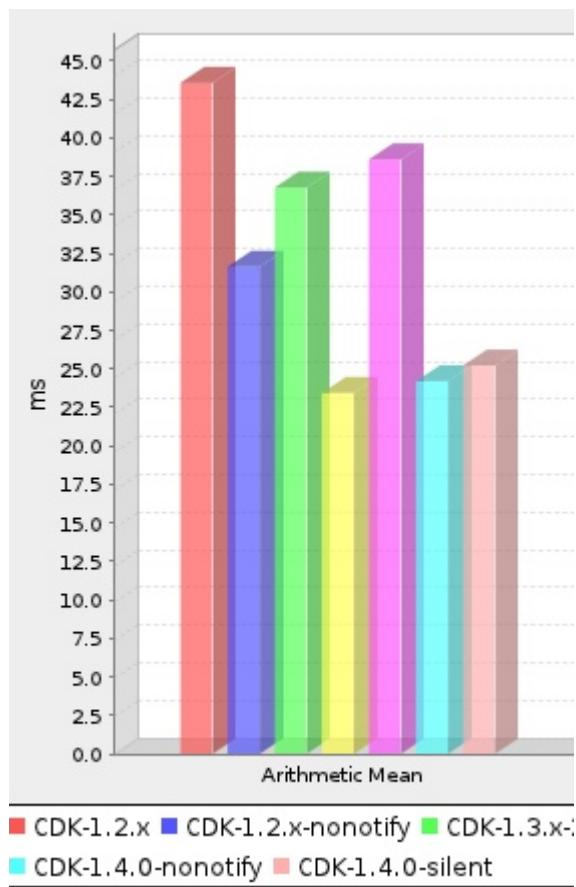
Red and blue are CDK 1.2.x (as the plot legend says), green and yellow the same for CDK 1.3.x (and both clearly faster than the 1.2 series, and purple an light blue the same for CDK 1.4.0. The last bar is the new silent module, a tid bit slower than nonnotify).
