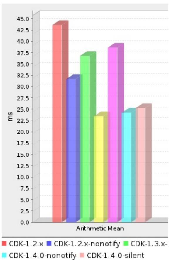
Red and blue are CDK 1.2.x (as the plot legend says), green and yellow the same for CDK 1.3.x (and both clearly faster than the 1.2 series, and purple and light blue the same for CDK 1.4.0. The last bar is the new silent module, a tad bit slower than nonotify.
