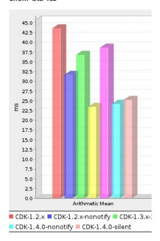
Red and blue are CDK 1.2.x (as the plot legend says), green and yellow the same for CDK 1.3.x (and both clearly faster than the 1.2 series, and purple an light blue the same for CDK 1.4.0. The last bar is the new silent module, a tid bit slower than nonotify.
