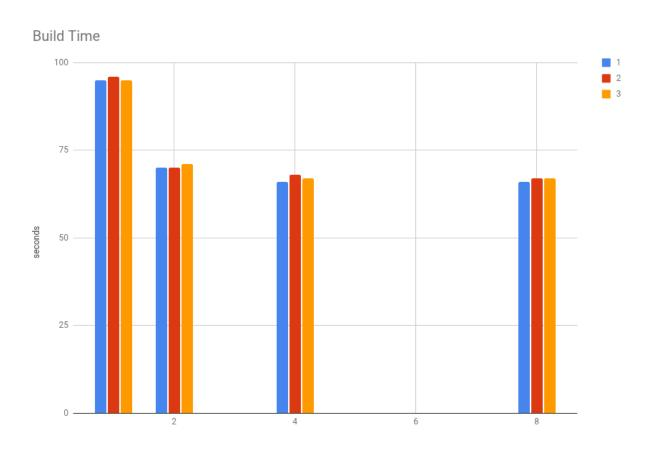
Going from one to two threads certainly pays of, but going to 4 shows only a three second speed up. The four processor cores were not utilized 100%, so I also attempted 2 threads core, but that showed zero improvement.
